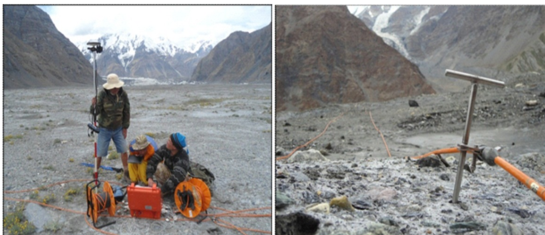
Figure 2.2.2.2. Vertical electrical sounding GeoTom-MK1E100 and differential DGPS ProMark-3 (rover station). Electrode and multi-core cables are shown on the right picture
